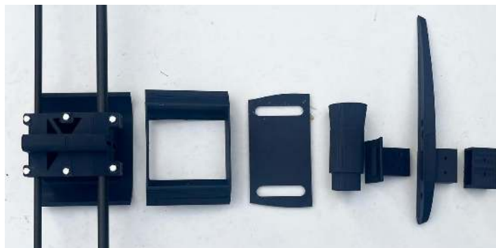
Figure 5.2: 3D printed joints and fixtures
