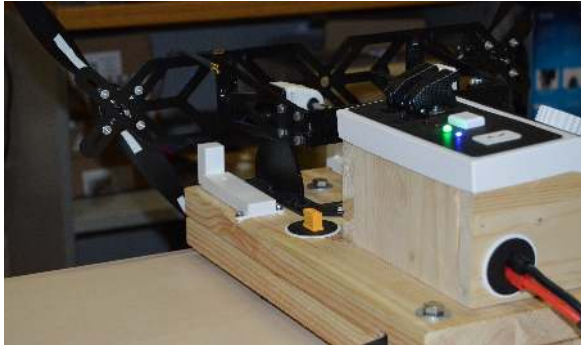
Figure 6.1: Propeller-mounted reflective target and IR sensor alignment for real-time rotational speed measurement.
