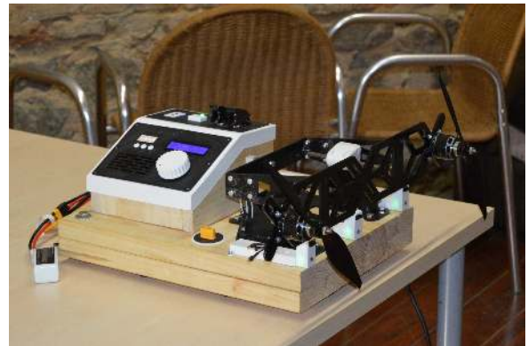
Figure 6.2: Twin-engine configuration demonstrating the bench’s dual-motor simultaneous measurement capability.
